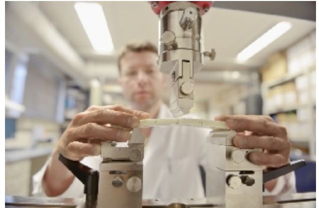
Three-point bending test on a CIPP-Liner
